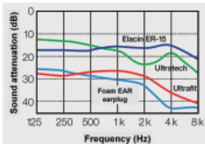
Figure 9: Attenuation curves of different earplugs
