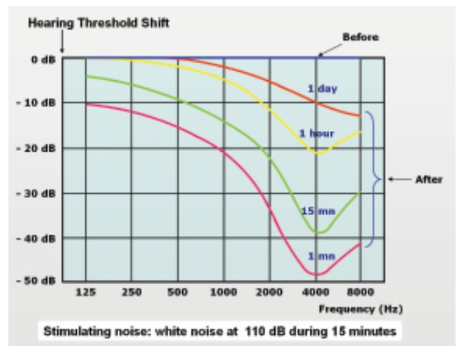
Figure 8: After exposure to loud noise the hearing sensitivity will be affected by a temporary threshold (TTS)
