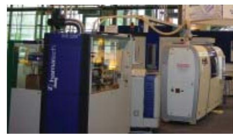
Considerable progress have been made to reduce the noise of CD and DVD replication line with the help of electric injection machine. With this modern DVD line noise level should be around 78 dB. (Picture JJ Wanègue)
